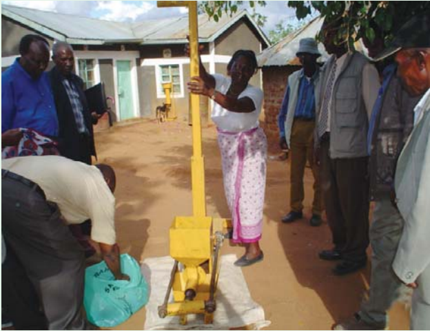
Kitui project on sunflower production and utilization integrated with bee-keeping: manual sunflower oil press
