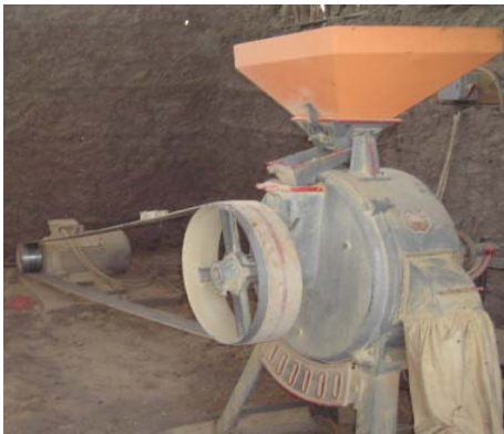
Plate 2: Normal flour mill used for Prosopis pod crushing
